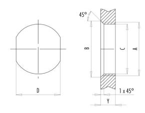
Installation direction: o-ring sits on chamfer.
